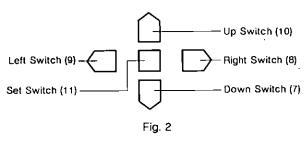
Up Switch(10): The cursor moves upwards.
