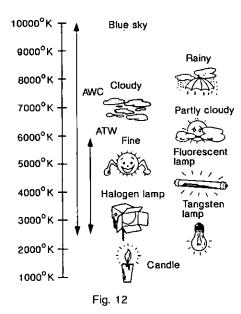
The white balance control can be chosen between the auto-tracing white balance (ATW) and one-touch automatic white balance control (AWC) mode by this menu.
