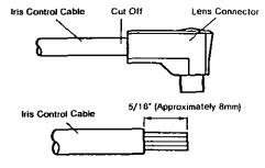
(2) Cut off the inner cable covers of the iris control cable as shown in the diagram.
