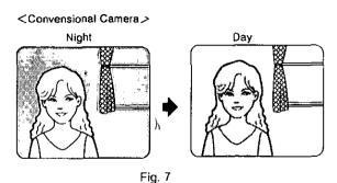
However, by using the WV-CL350 in the preset "OFF" mode, it is possible to compensate for difficult lighting conditions. In this mode, the picture is divided into 25 zones or mask areas. It is possible to mask (or tell the camera to ignore) any bright light sources in those mask areas that might interfere with picture clarity.
